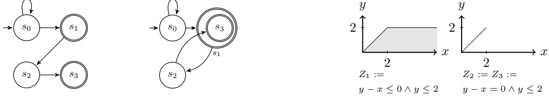
Figure 3. Taken from [18]. Consider the TA obtained from the PBTA in Fig. 1, by setting p = q = r = 2 . The symbolic state space \mathcal{PZG}(\mathcal{B}) of this TA, with \ell_1 \in F , contains 4 states (shown on the left): s_0, s_1 = (\ell_1, Z_1), s_2 = (\ell_2, Z_2) and s_3 = (\ell_1, Z_3) . Note that there is no accepting cycle. The graphical representation of the zones Z_1 – Z_3 (right) reveals that Z_3 \subseteq Z_1 and hence s_3 \sqsubseteq s_1 . As s_3 \sqsubseteq s_1 and both are reachable, the subsumption abstraction might map \alpha(s_3) = s_1 , introducing a cycle s_1 \Rightarrow s_2 \Rightarrow s_1 in \mathcal{PZG}_\alpha(\mathcal{B}) .
